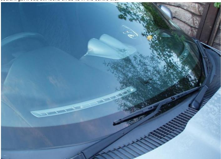
The cloth covered bits with the vents in them are simple, the cloth covered part is held in with 2 clips (see pic below) - at the front and back of the right side. Just CAREFULLY push a screwdriver in here and pop the clips, the whole thing will lift out. The vent is held in one Phillips screw, undo this and it just pops out. Zoom in on the pic below as my notes are quite small.
