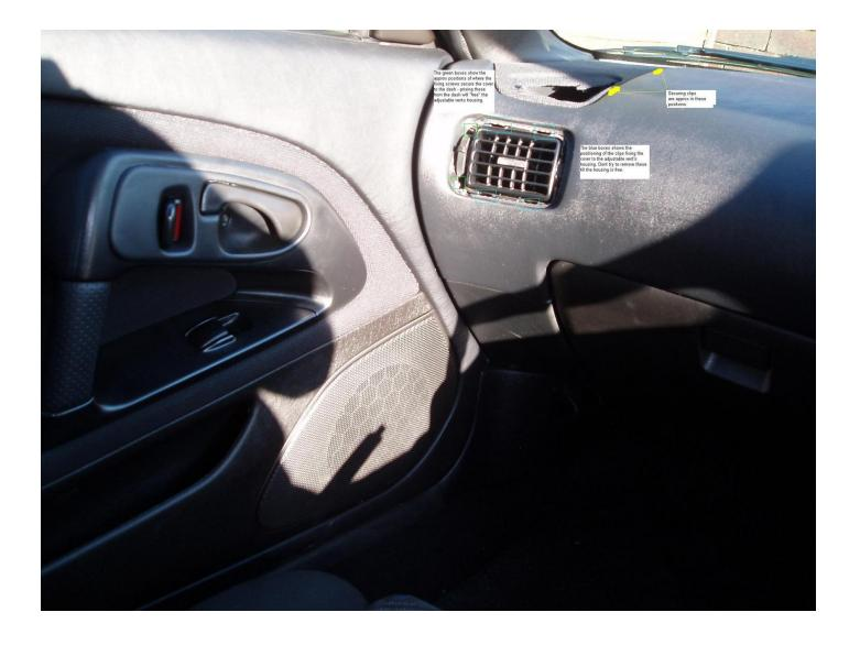
The adjustable vents were the most difficult as i was terrified of breaking them. The thing is they assembled this from the inside. The air tube? with the adjustable vent fixed on the front of it has been offered up to the rear of the dash, the cover (which we want) was then placed on the front and clips onto the adjustable vents housing (see on the pic above) ....then to make double sure they screwed the cover on from INSIDE the dash
